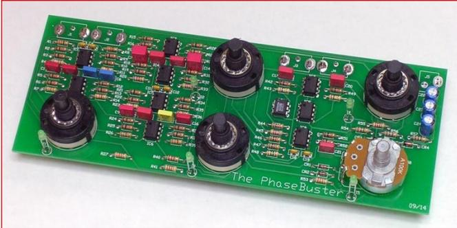
The only hand wiring consists of three short, bare-wire jumpers between the VARIABLE pot and the board. Almost all the components, including the rotary switches, are on one side of the board; the input, output and DC power connectors are mounted on the rear.
