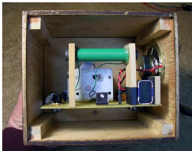
The vernier dial mechanism came from a ham radio flea market and dates to the late 1930s. Its linear 'logging' scale was replaced with one that carries actual AM-band frequencies.
