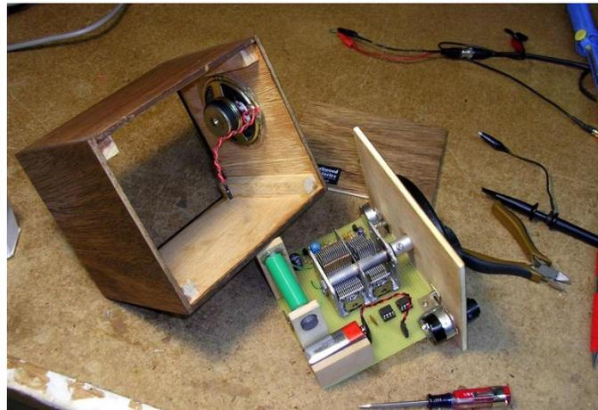
It uses a variable capacitor scavenged from an old "All-American Five" table radio, and a home-wound antenna with about 60 turns of hookup wire around a hunk of ferrite material. The inductance was chosen to resonate just below 520kHz with the tuning capacitor fully-meshed. A small trimmer cap, C2, sets the top of the dial to about 1730kHz.
