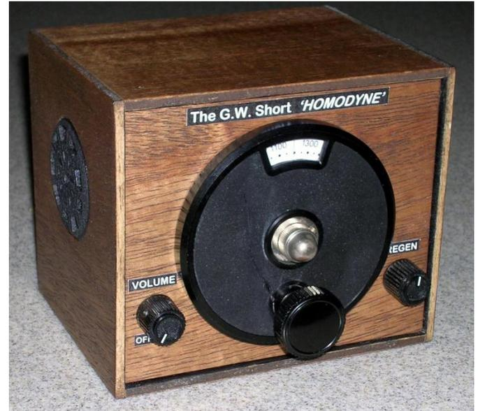
The front and rear panels actually form a 'sandwich,' and the radio is held in its box with only one screw through the back:
